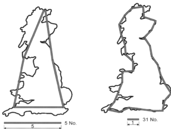
Fig.1. Coastline of Britain measured by two different length measuring sticks
