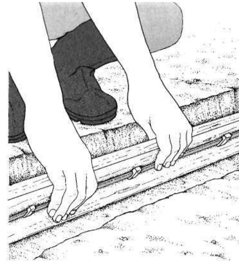
Cables laid underground should be protected against accidental damage while digging. Cover the cable with a treated plank or place tiles over it.
