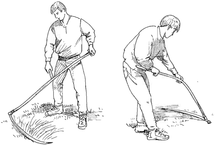
FIGURE 7.1. The ergonomically correct use of tools provides long-term benefits to our health, comfort, and well-being while gardening. The design of tools such as scythes has a huge impact on the way we use our bodies and our perception of what kind of work we like to do. Lightweight European scythes (left) have straight handles, allowing you to keep your back straight during use. Heavy American scythes (right) force the user to bend forward, slowly destroying the spine's integrity. Guess which one is more pleasant to use for long periods. Guess why Americans don't use scythes very much.
