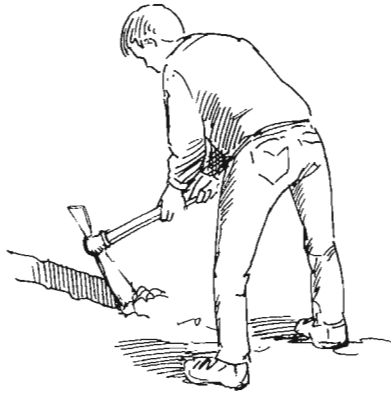
Mattock, two heavy blades, one parallel to handle, one perpendicular
