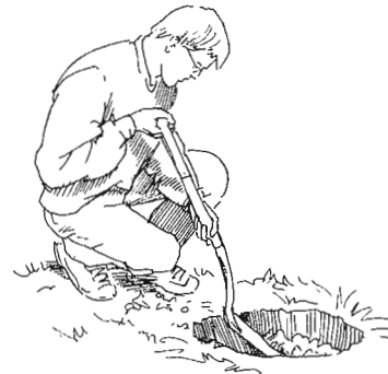
FIGURE 7.2. A proper shoveling stance keeps your back straight at all times and uses your legs, your arms, and the levering action of the shovel to do the work. When working in a deep hole or with a D-handled shovel, squatting is the best position, as shown here. Long-handled shovels should be used when standing fully upright.
