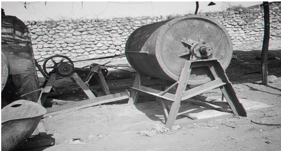
Figure 3: A ball mill being used as part of a gold mining operation in Arequipa, Peru ©Practical Action
