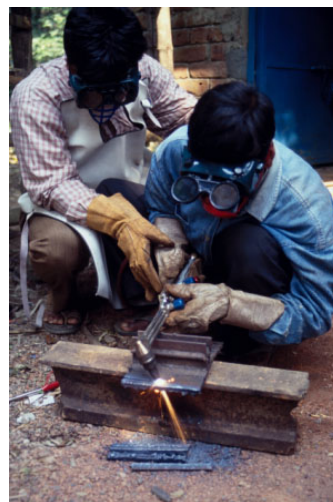
Figure 4: Flame cutting. Practical Action organised training for Asaduzzman Munshi in welding. As a result he has now started a small metal workshop of his own, earning Tk 3000 monthly (2000). In the process of cutting parts for a three-wheel rickshaw structure.
