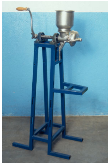
Figure 5: A large hand grinder produced by Practical Action Southern Africa.
