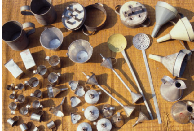
Figure 2: Examples of the some of the tin products produced by the trainers who carry out training in tinsmithing by Practical Action Bangladesh.
