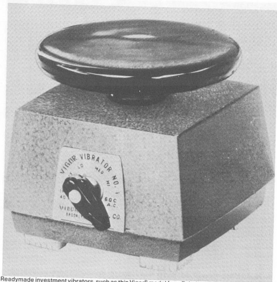
Readymade investment vibrators, such as this Vigor® model from B. Jadow and Sons, Inc., are also available to jewelry workers.
