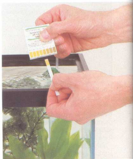
Above: Taking regular readings of pH value is very easy with modern test kits. Here, paper strips treated with an indicator provide instant results. Other kits use liquid reagents added to a small sample of tank water.
