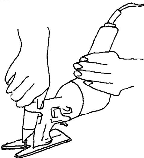
Electric drill with jig saw attachment
