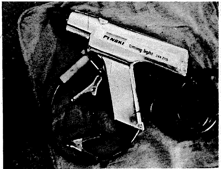
The power timing light emits a very bright flash and is more accurate and easier to use than the simple neon bulb light.
