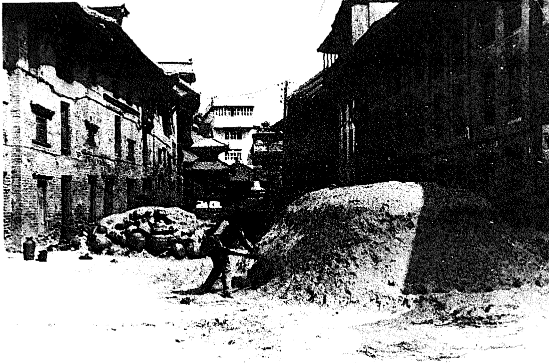
Fig. 2-4: Straw-fired kiln in Thimi, Nepal
