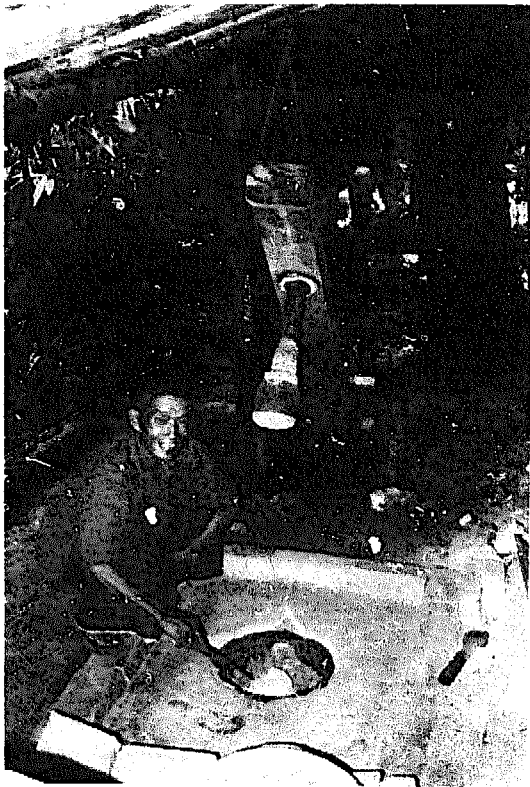
Fig. 1-8: A manual hammer for grog crushing
