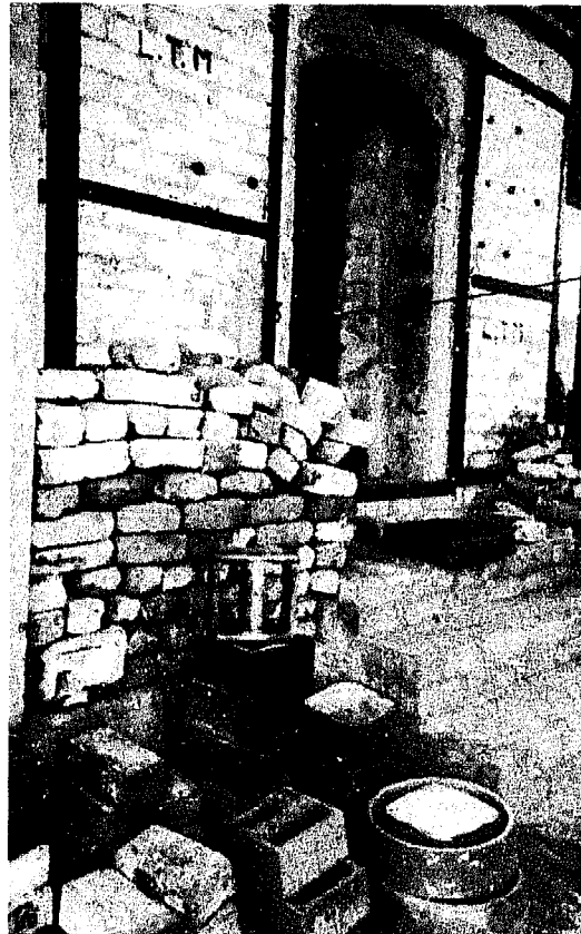
Fig. 1-45: The hollow spaces of these firebricks are filled with rice husk ash. A prototype of a low thermal mass kiln developed at the Khurja Centre is seen behind the bricks.
