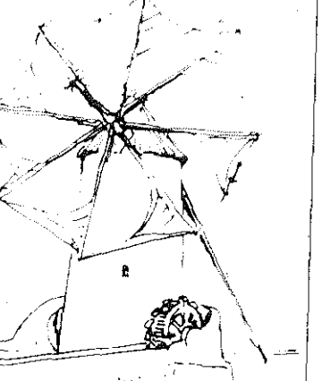
Rigging of Murcian mill. This one has a frame for reefing sails.
