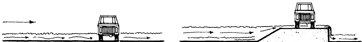
Figure 13.7a An embankment drift in a stream with deep water flow because of slight gradient will create a shallow rapid flow across the top of the drift.
