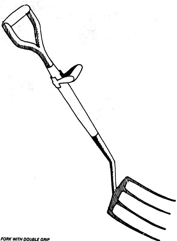
People having difficulty holding a fork, can facilitate gripping with an extra grip half-way the bar. This way the fork can be managed better. The rear grip is also fixed onto the bar in a comfortable position for the hand.
