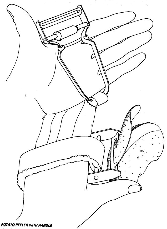
If you lack the strength in your hand to hold a potato peeler steadily, you can attach a handle to the peeler.
