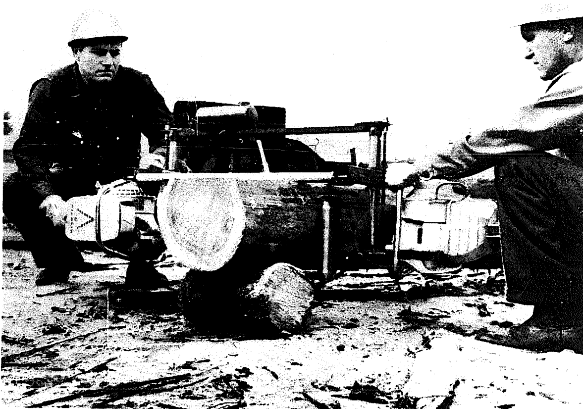
Granberg Alaskan Mill in operation
