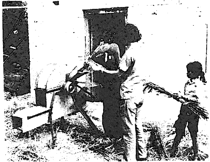
Threshing machine, driven by a small water turbine.
