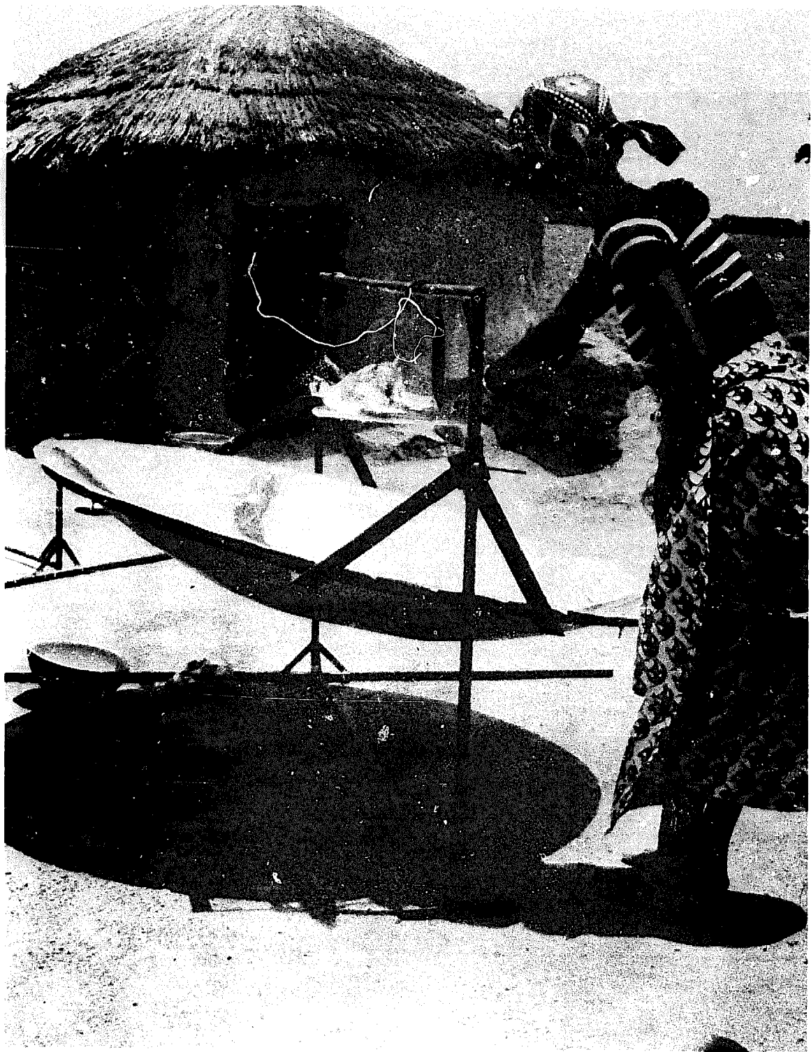
Figure 28. Photograph of Solar Cooker Developed by Danchurchaid Being Used to Broil a Chicken in a Village Near Pô, Upper Volta.
