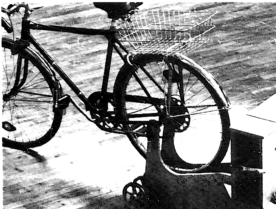
FIGURE 75 The Bik-O-Generator will power a grain mill or generate electricity. A pulley attached to a power take-off wheel could be attached to many other belt-powered tools as well. (Reprinted from Pedal Power © 1977. Permission granted by Rodale Press, Inc., Emmaus, PA 18049)
