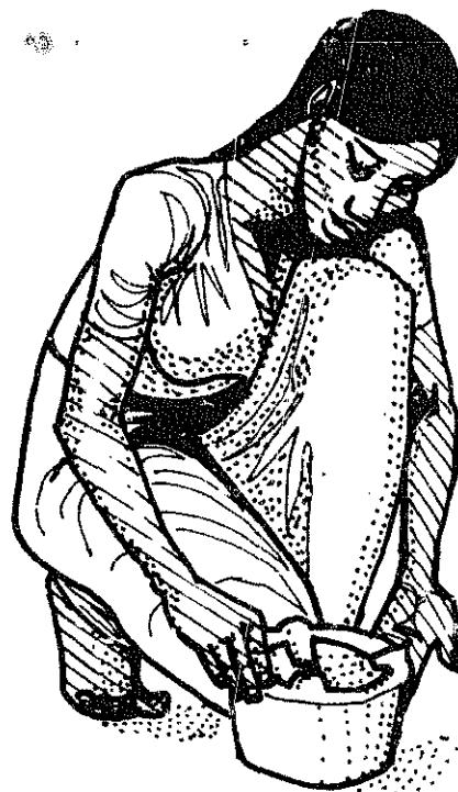
Pot rests are joined to the second pot seat and tunnel entrance removed
