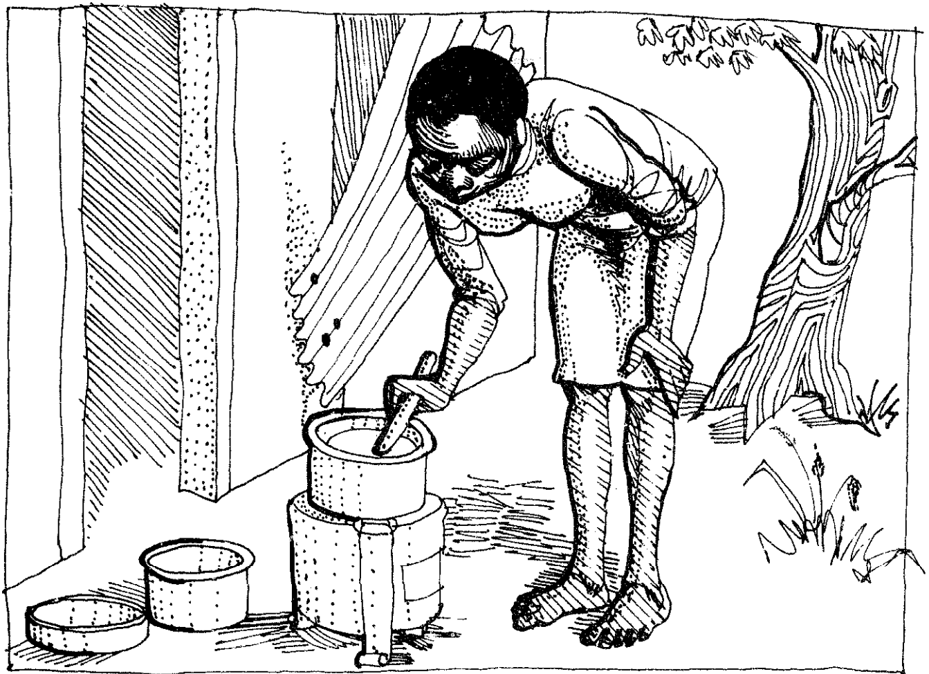
25. CEMENT/VERMICULITE-LINED STOVE (KENYA)
