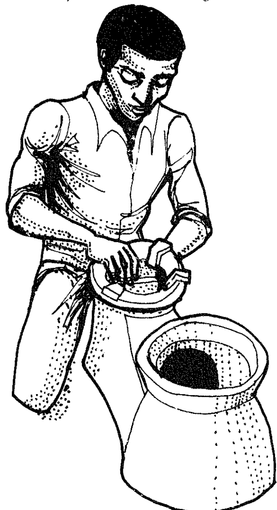
The three pot rests are attached to allow smoke to escape
