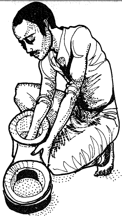
The other side is joined and smoothed together
