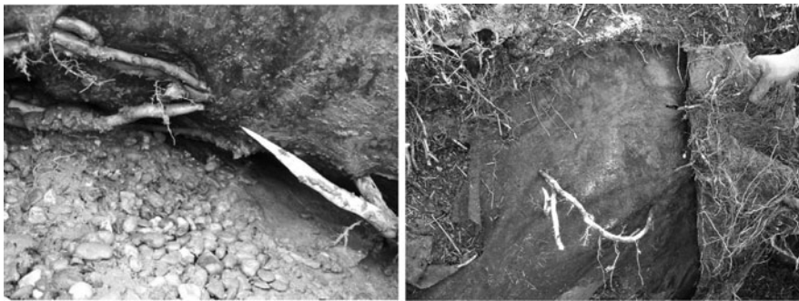
Fig. 9.6 Roots and rhizomes of Phragmites australis puncturing LDPE liner at the base and side of the reed bed
