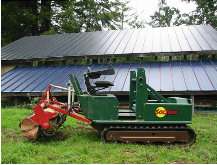
Fig. 7.1 Solar charged electric agricultural tractor designed and built by Stephen Heckerth, www.renewables.com
