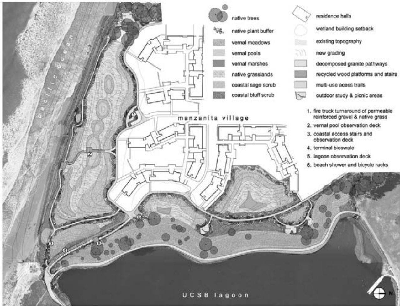
Figure 4.66 The master plan for the lagoon included vernal meadows, pools, and marshes as well as native grasslands, native trees and plantings, and coast sage scrub and bluff scrub. Image courtesy Van Atta Associates.
