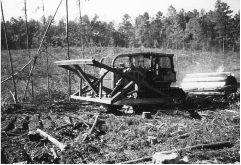
Figure 6.1. Roller chopper used for site preparation in east Texas forest. This treatment breaks up the woody debris and roughens the soil surface to facilitate and improve planting success.
