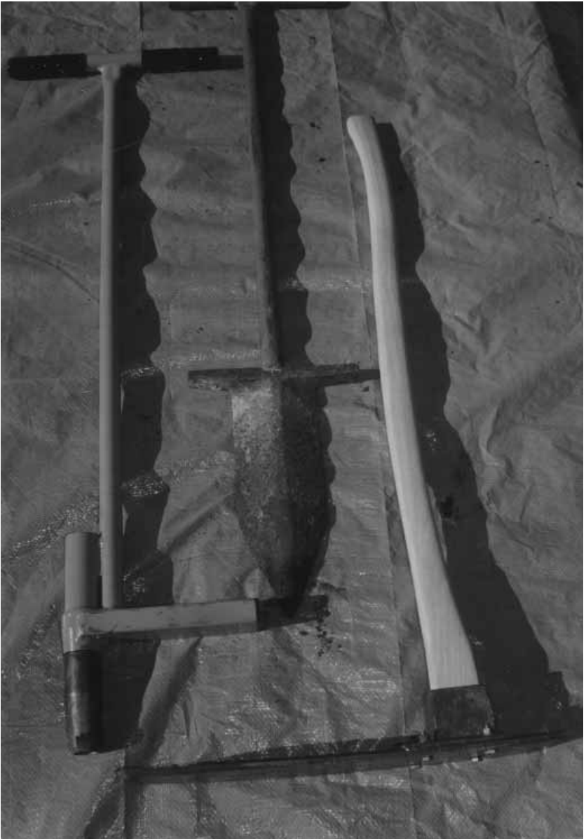
Figure 7.5. Hand implements designed for transplanting seedlings into wildlands. Seeding dibbles (left) remove a soil core for the seedling to be planted into. KBC bars (middle) are most appropriate in rocky soils that are difficult to penetrate. Hoedads (right) are used to create a small planting pit.
