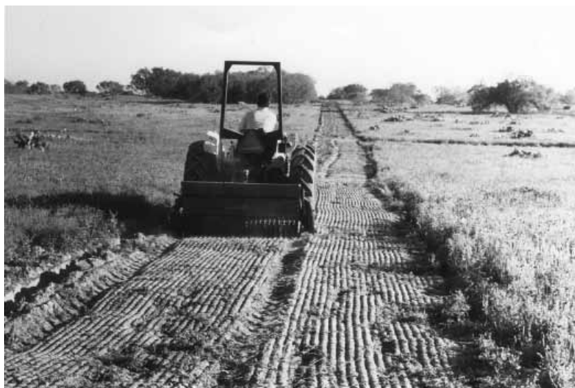
Figure 7.4. Cultipacker-type seeder operating on recently plowed strip in south Texas. This equipment creates many small depressions but requires a well-tilled seedbed.
