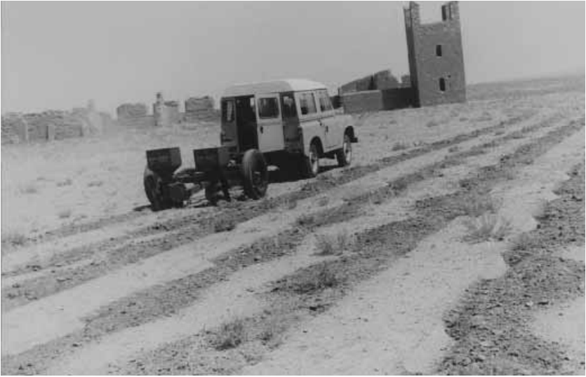
Figure 7.3. Kimseed camel pitter creating and seeding pits in a bare, crusted soil. Water harvesting approaches can greatly improve seedling establishment in this situation. Photograph courtesy of Australian Revegetation Cooperation.
