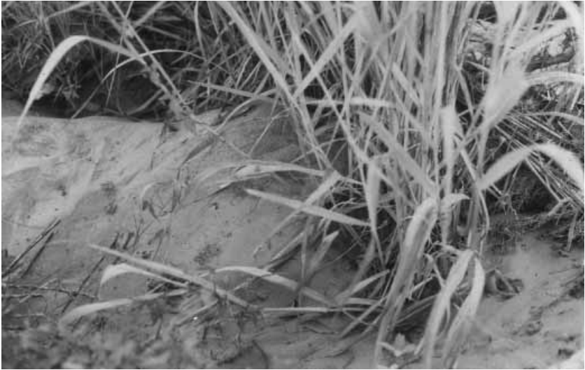
Figure 3.6. Single switchgrass ( Panicum virgatum ) plant transplanted into actively eroding channel near College Station, Texas, trapped organic materials (upslope) and about 13 cm of soil (downslope) within 60 days.
