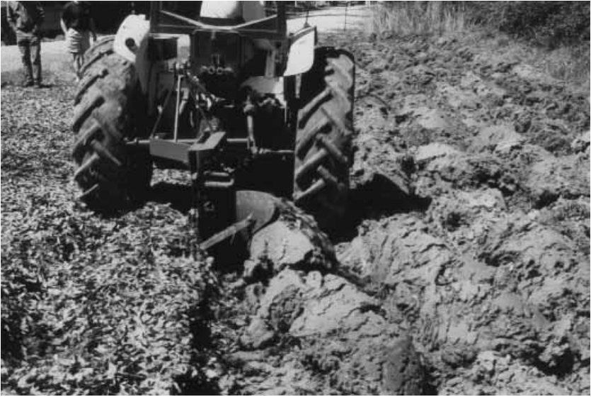
Figure 6.3. Moldboard plow used to loosen compacted soil and incorporate leaf litter into an old roadbed.
