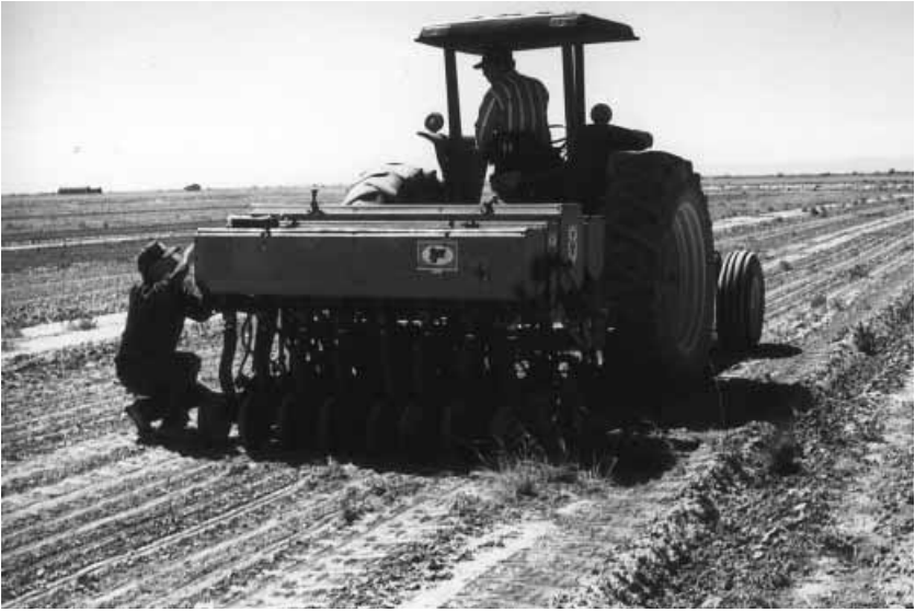
Figure 7.1. Rangeland drills are able to operate in rough terrain and can plant smooth and fluffy seed simultaneously. They create small furrows for each row, plant seed at controlled depths, and firm soil over the seed.
