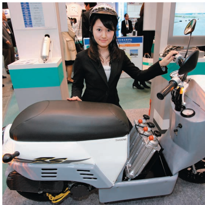
Figure 13.15 Hydrogen fuel cell application. A small hydrogen-powered fuel cell powers the scooter pictured here. (Yoshikazu Tsuno/AFP/Getty Images)
