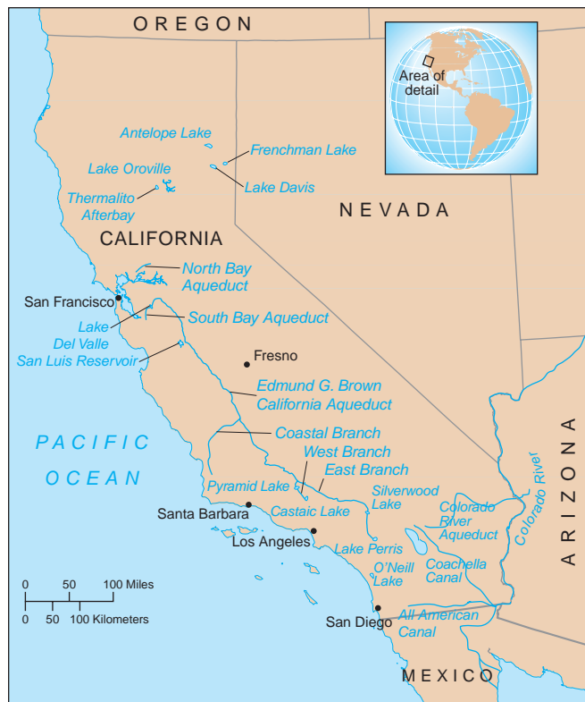
Figure 14.23 Water diversion in southern California. Largely desert, southern California relies on water diversion for the water needs of its millions of inhabitants. The California Water Project includes 1042 km (648 mi) of aqueducts to transfer large quantities of water to southern California. This map also shows some of the main reservoirs of the California Water Project.
