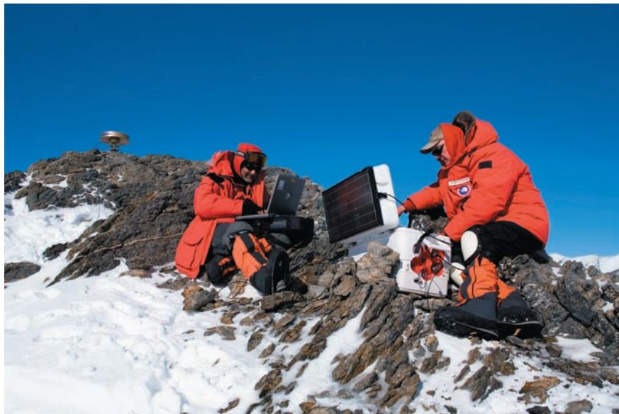
Figure 16.9 Research in Antarctica. Scientists set up a GPS receiver in West Antarctica as part of the West Antarctic GPS Network (WAGN) project. The WAGN project is measuring crustal movements surrounding the West Antarctic Ice Sheet. These movements in the lithosphere could affect the future of the ice sheet and its corresponding effect on sea level. (Bryan & Cherry Alexander Photography/Alamy)
