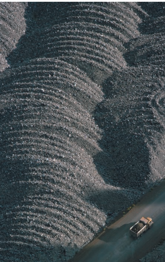
Figure 16.5 Aerial view of gold tailings. These tailings are stacked in long, parallel mounds. The truck at the lower right gives a sense of scale. Photographed near Yankee Fork of the Salmon River, Idaho. (©Natalie Fobes/©Corbis)
