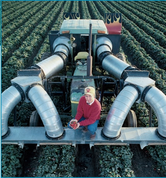
Salad-vac. This machine controls certain insect pests without the use of chemical pesticides. Photographed in Salinas, California. (Richard Steven Street/Streetshots)
