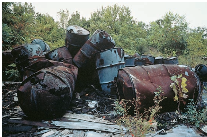
(a) Hazardous waste in deteriorating drums at a site near Washington, D.C. The metal drums in which much of the waste is stored have corroded and started to leak. Old hazardous waste dumps are commonplace around the United States. (Courtesy USDA)
