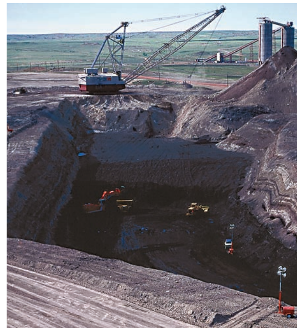
Figure 11.6 Surface coal mining. The overlying vegetation, soil, and rock are stripped away, and then the coal is extracted out of the ground. Photographed near Douglas, Wyoming. (Kristin Finnegan Photography)
