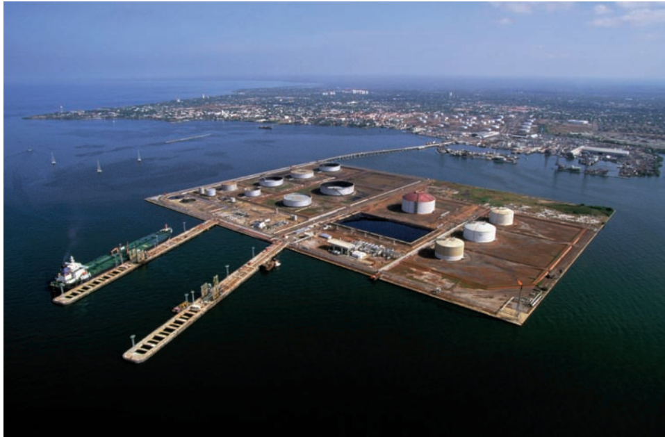
Figure 22.13 Lake Maracaibo, Venezuela. Drilling platforms are located throughout the lake, and pipelines join the oil wells to refineries on land. Shown are storage and export facilities in the foreground and the town of Cabimas in the background. An oil tanker is docked at the leftmost pier. (© Yann-Arthus-Bertrand/©Corbis)
