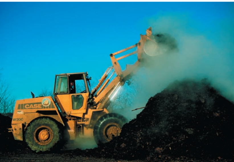
Figure 24.6 Municipal solid waste composting. This pile of partially decomposed compost is curing (maturing) at outdoor temperatures. Photographed in Glen Rock, New Jersey. (©Alan L. Detrick/Photo Researchers, Inc.)
