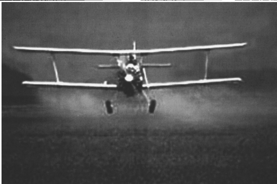
Fig. A.11: Aerial spraying is advantageous particularly over large areas, in tree plantations or if the land is too wet. Courtesy: "The US Environmental Protection Agency" and "International Network for Environmental Compliance and Enforcement". With permission from the office of the INECE Secretariat, Washington, DC.
