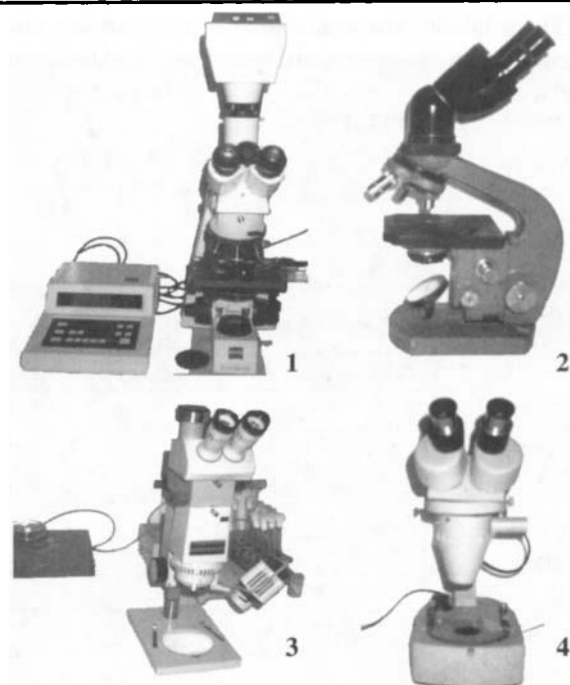
Fig.M.12: Types of microscopes: 1. Phase contrast microscope, 2. Research microscope, 3. Dissecting microscope, and 4. Stereoscopic microscope.
