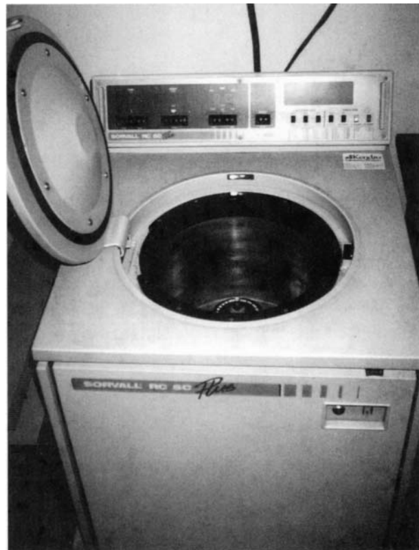
Fig. C.20: A cooling, high-speed centrifuge.
