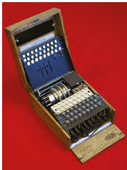
Fig.2. (above) The German Enigma machine, used to encipher messages sent by the German Army, Air Force, Navy and Secret Service, (right) a Lorenz machine, used to encrypt messages sent by Hitler and the high command. Colossus was developed to speed up the breaking of these cipher systems. (Both images courtesy of Bletchley Park, copyright mubsta)
