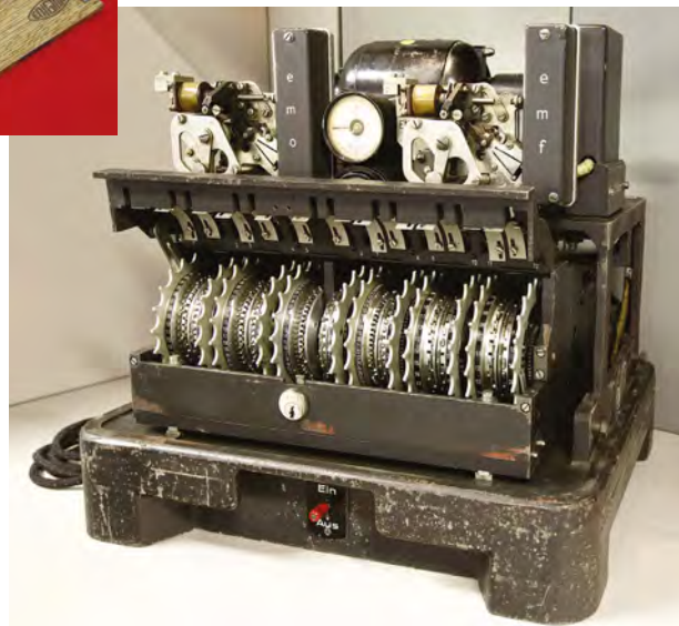
Fig.2. (above) The German Enigma machine, used to encipher messages sent by the German Army, Air Force, Navy and Secret Service, (right) a Lorenz machine, used to encrypt messages sent by Hitler and the high command. Colossus was developed to speed up the breaking of these cipher systems. (Both images courtesy of Bletchley Park, copyright mubsta)
