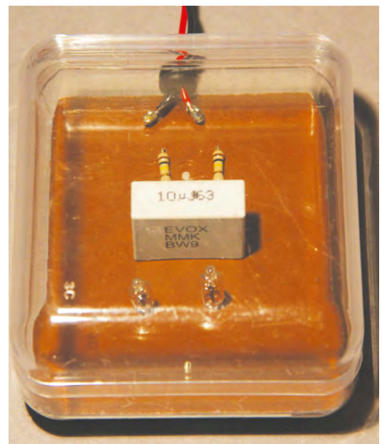
Below – Views of a neon lamp multivibrator built into a small plastic container. These photos with the neon lamps illuminated are with the lid removed
