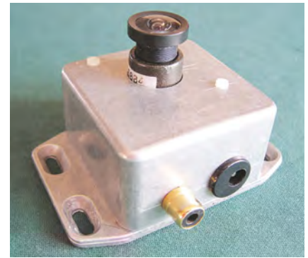
Fig. 2. The diecast box sealed ready to be put in position
