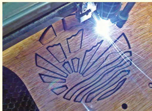
Fig.17. Laser cutting the retro-design radio enclosure
