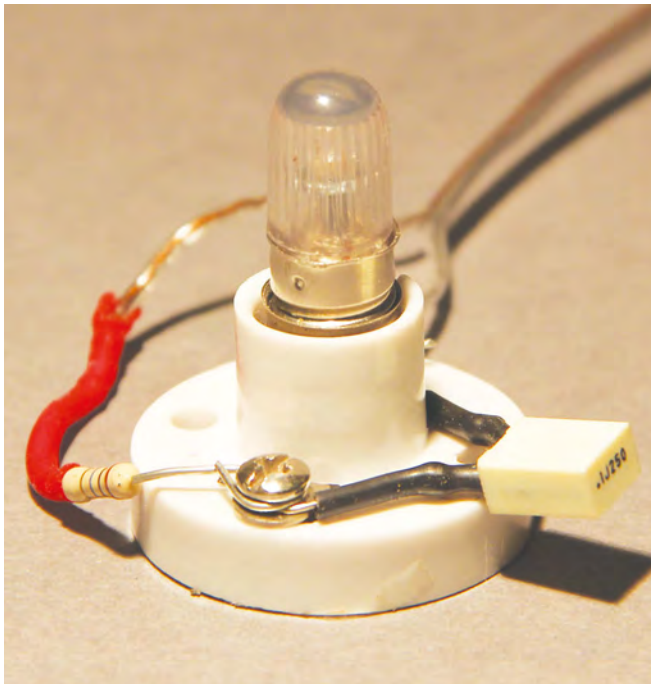
Left – Neon relaxation oscillator using an MES neon lamp and components wired directly to the MES lamp holder. (Note: the lampholder is normally rated at 50V maximum, but the neon works between 50-60V. Be aware that voltages above 50V are not considered safe and any exposed metal should be insulated. The units shown should be assembled into a suitable box. Although, in this case, the high voltage side of the resistor is sleeved and any current flow from the resistor is limited to a safe value, there might still be a possibility of a high current pulse from the capacitor.)
