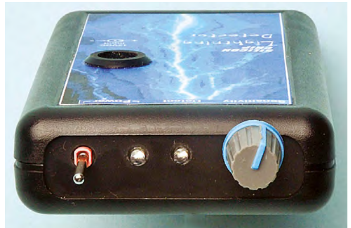
This end-on view shows the two controls and two LEDs which mount on the end panel
