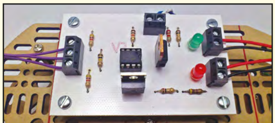
DC Motor Controller PCB in-place on the buggy chassis
