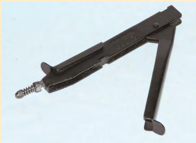
Fig.3. A hand nibbler can quickly cut through most thin sheet materials. A tool of this type can be used to produce large cut-outs very quickly, but it cannot be used to make curved cuts
