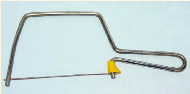
Fig. 1. A coping saw is relatively inexpensive, but can be used to make cut-outs of practically any size or shape. This one is fitted with a tension file blade
