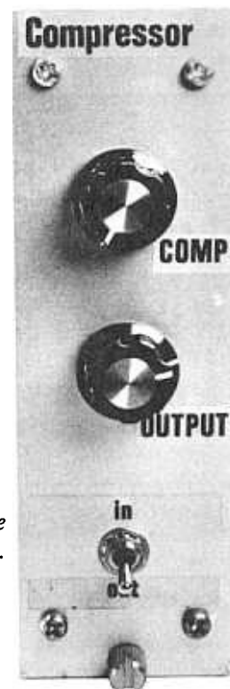
Figure 5-45 Compressor mounted in a Vector-Pak card module prior to installation in the pedalboard project (No. 23).
