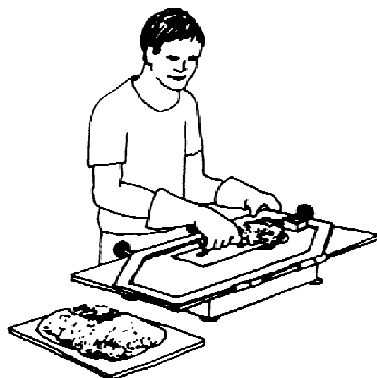
Figure 2: Work the mortar mix under vibration
