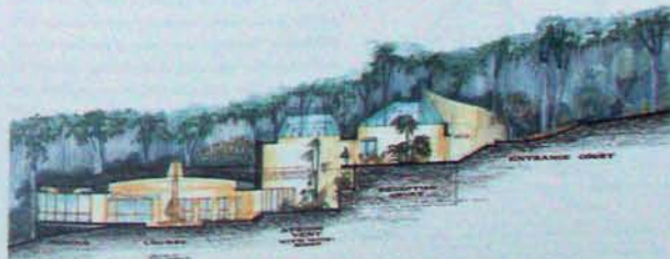
Figure 8.5: An earth-clad residence with a wind scoop that functions as a thermal chimney (Sydney, NSW, Aust.). Architects: ICA Space Design Pty Ltd.
