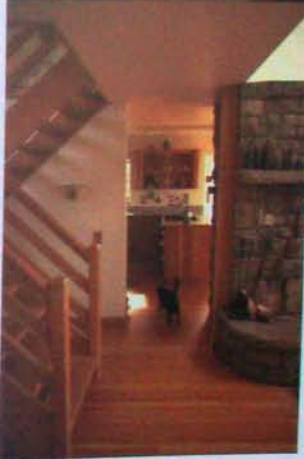
Left: This residence in British Columbia, Canada, has all natural finishes. The rock wall acts as a thermal-storage element and is used in conjunction with a minimal-emission wood-burning enclosed-combustion stove. (Photograph: B. Phoenix)
