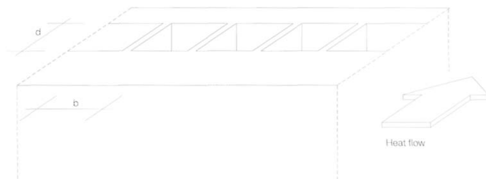
2.6.14 Small or divided non-ventilated voids (air spaces)
