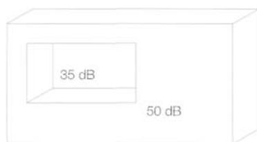
2.6.95 Resulting sound reduction index R_{w, R, res} (dB) in relation to sound reduction index of wall, sound reduction index of window and its proportion of the area (%)
