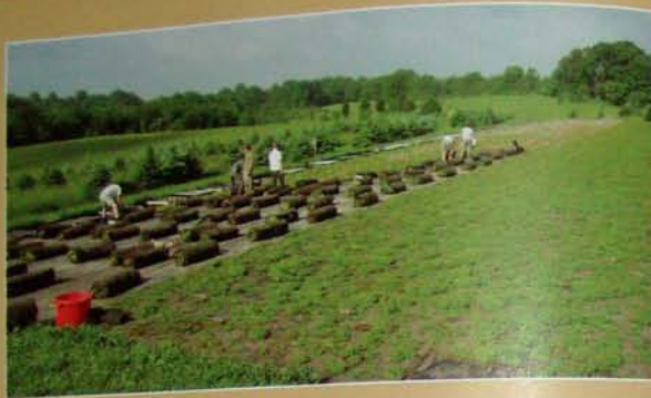
Right: Plants are grown directly in Enkarooof VM and transported to the site, ready to unroll.
