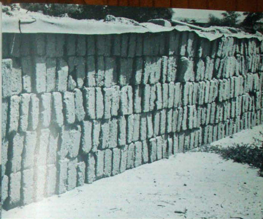
Fig. 7.3 Adobes stacked. Note that to minimize breakage, adobes are stacked on edge, not flat. Tarpaper on top protects bricks until used. Chipped corners and ragged edges won't hurt a thing.
