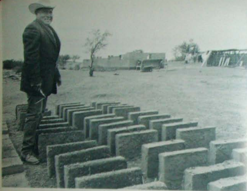
Fig. 1.1. Papago Indian Reservation today. Standing adobes vertically speed the curing process. Later, these will be moved to homestead in background.
