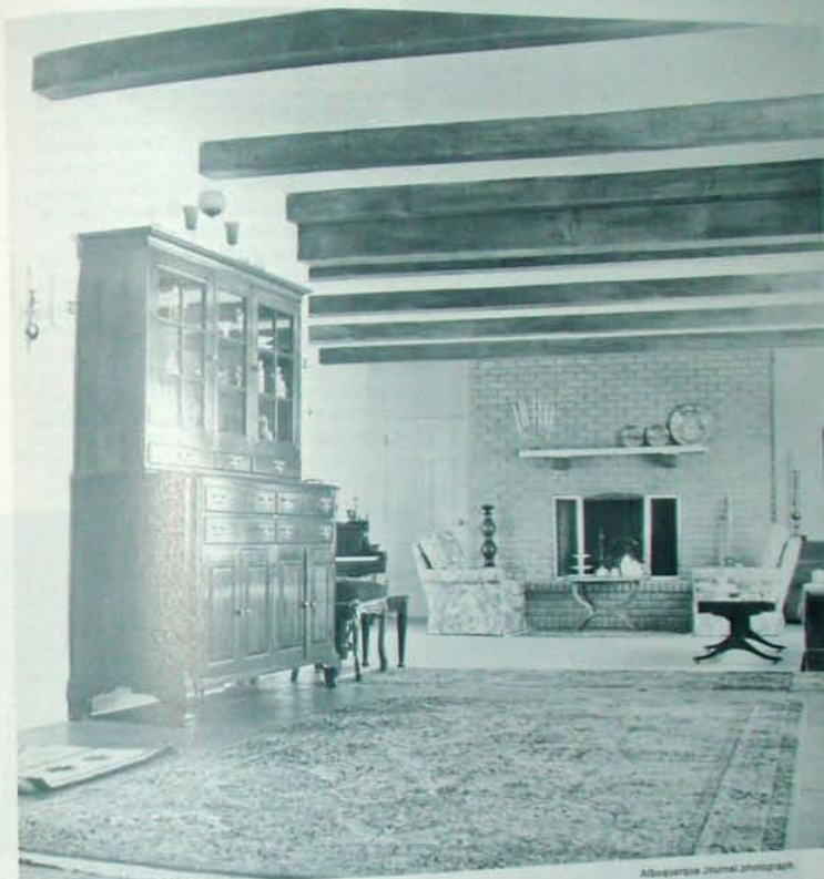
Fig. 18.2 Residence, Placitas, New Mexico. P. G. McHenry, Jr., architect-builder. New bricks antiqued by tumbling in a concrete mixer soften the sometimes harsh lines of a brick-faced fireplace.
