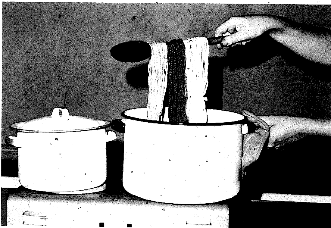
Skeins are lifted from pot or dyebath after being treated with different mordants and yield different color shades as a result. The yarn at left was treated with alum; the center, chrome; the right, no mordant.
