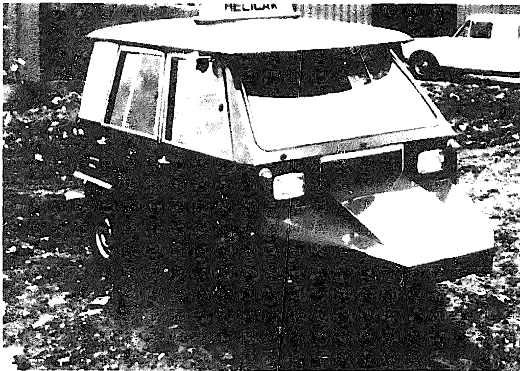
Urban taxi with 125cc engine and rust-proof fibreglass body, manufactured in Indonesia.
