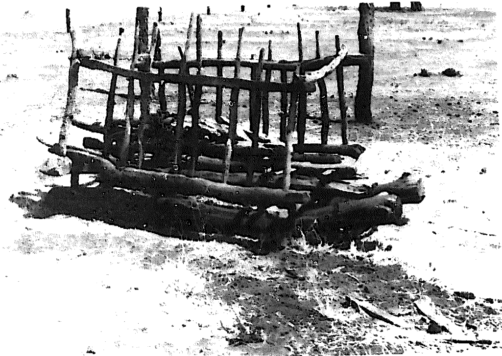
Ox sledge: Botswana. Even in a device as simple as a sledge there is scope for the improvement of traditional designs. Contrast the heavy, inflexible construction with the Philippine buffalo sledge.
