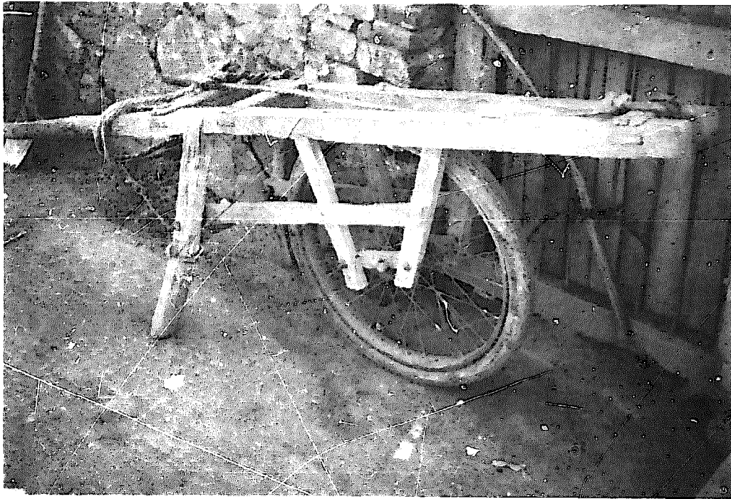
Chinese wheelbarrow with wooden frame. (Photo: J. Collett)
