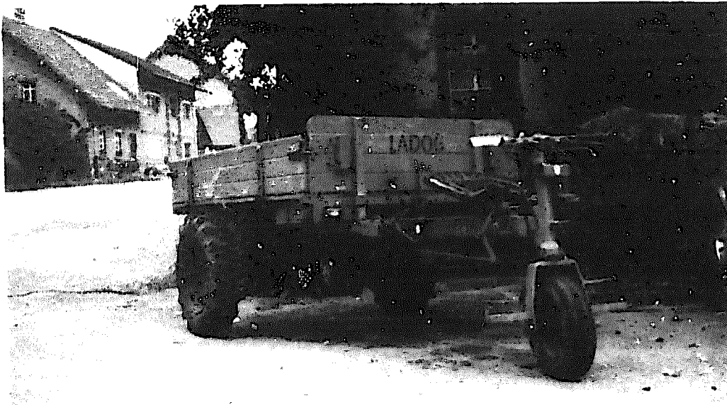
Three wheeled agricultural vehicle in Germany. As the engine is fitted under the body, it is unlikely to be removed regularly.
