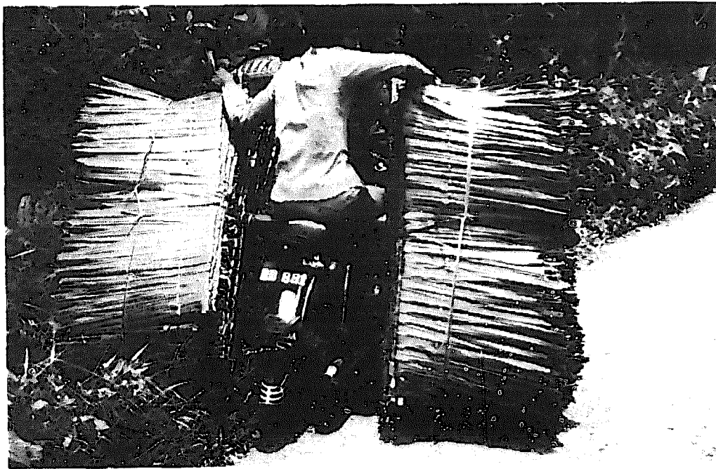
Surprisingly large loads can be carried on a motor cycle with a suitable load frame and careful packing. However, a load as large as this would be difficult to control on rough ground or busy streets.
