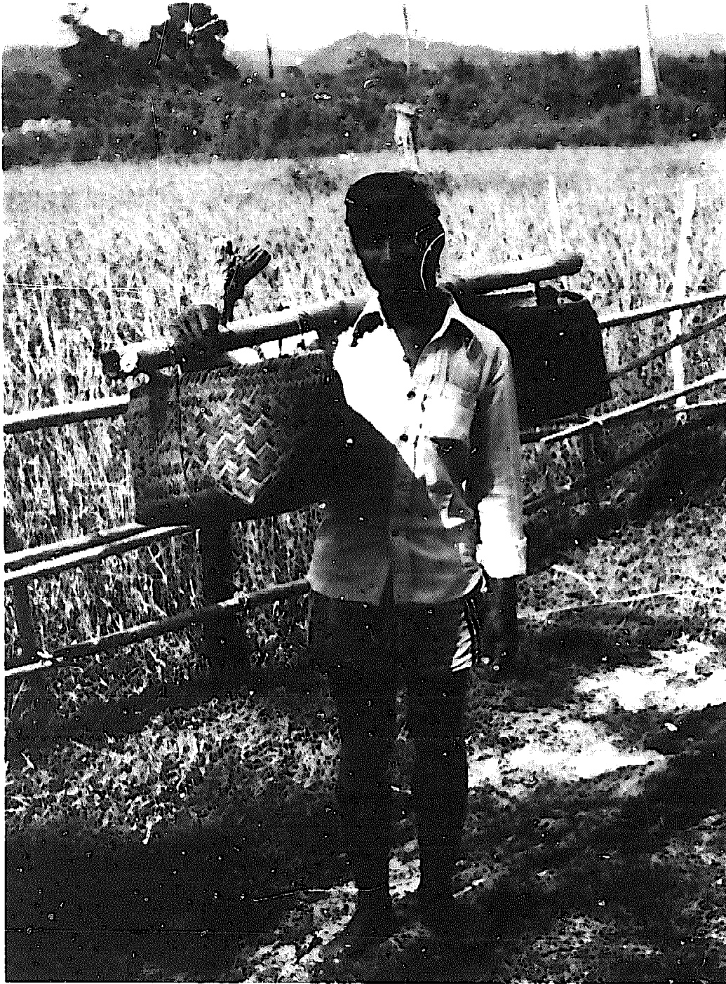
A rigid shoulder pole in Laos. This type of pole is easy to make from bamboo or timber, but it is not as comfortable to use as a flexible pole. The load is balanced and controlled with one hand.
