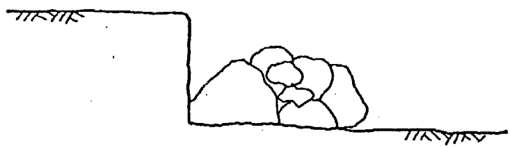
View B-B: Excavated section ready for loading
