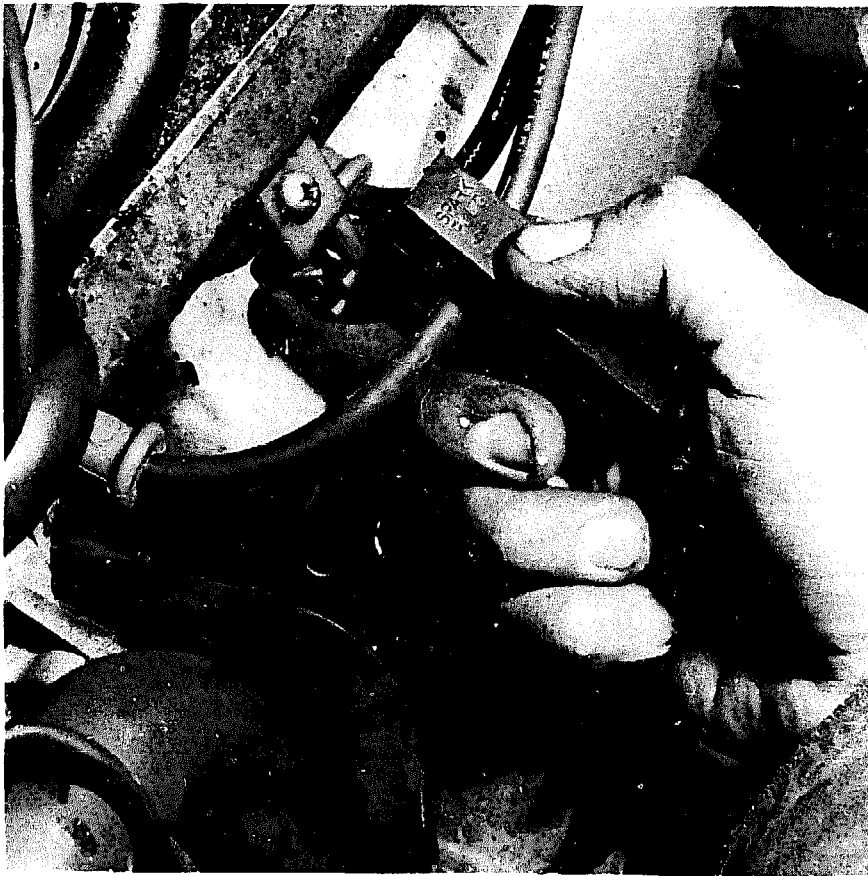
The third timing light lead has to be connected to the number one spark plug cable.
