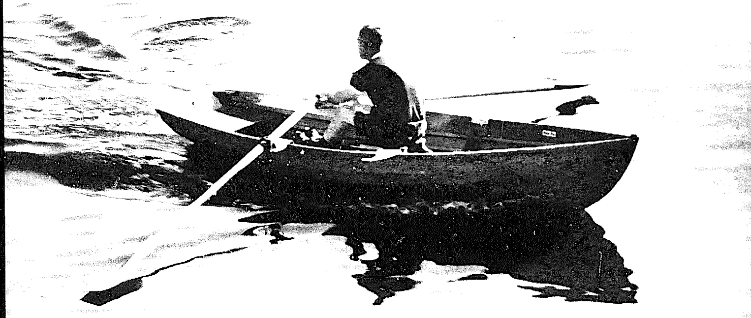
Above: A 13-foot Chamberlain dory skiff built by Thomas G. Plant, Jr., of San Francisco. This rowing model is fitted with a sliding seat and spoon-blade oars. Below: The same model dory skiff built by Plant and rigged for sail.
