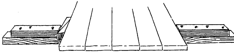
8(b). This wedge set-up may be used in lieu of cabinet clamps.
