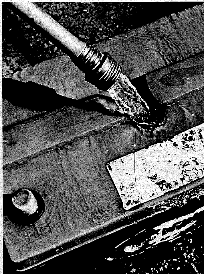
After washing, the battery should be kept clean and dry. After reinstalling the cables, lightly coat the tops of the terminals with petroleum jelly to prevent corrosion build-up.
