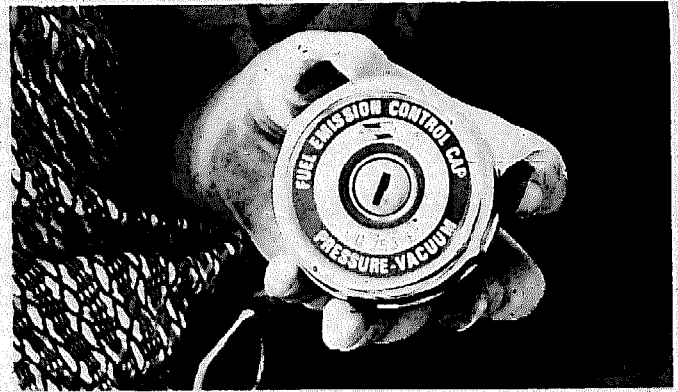
7 A special pressure vacuum filler cap must be used on all cars equipped with a fuel evaporative system.
