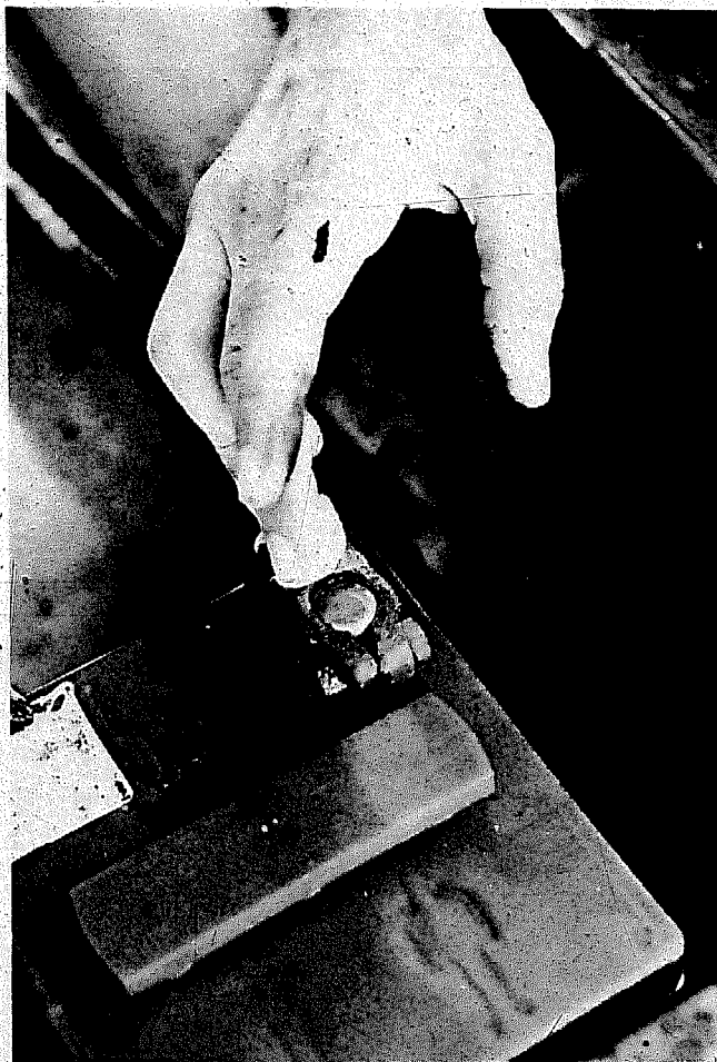
After washing, the battery should be kept clean and dry. After reinstalling the cables, lightly coat the tops of the terminals with petroleum jelly to prevent corrosion build-up.
