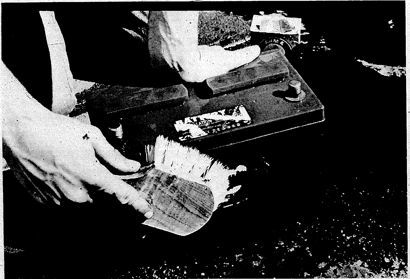
Periodic removal and washing of the entire battery with baking soda solution will prevent dirt from discharging the battery. The case should be thoroughly rinsed and dried before reinstallation.
