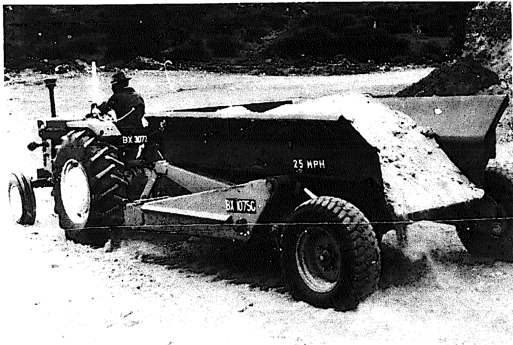
Figure 32. Small dump truck combination consisting of small tractor, towed chassis and hauling container (Southern Africa)
