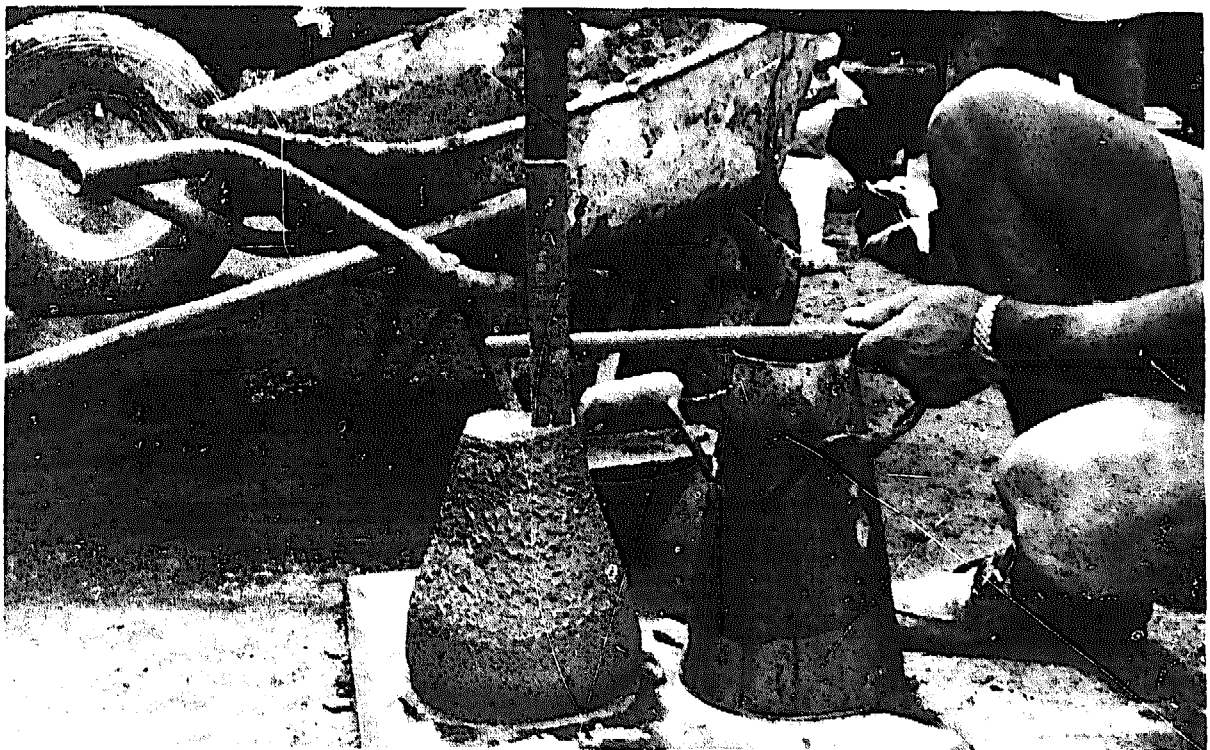
Figure 4-20. Mortar slump test
