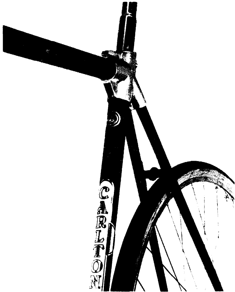
Figure 10.5 Carlton frame with carbon-fiber-reinforced plastic tubes and alumi- num lugs. Courtesy Raleigh Industries, Ltd.
