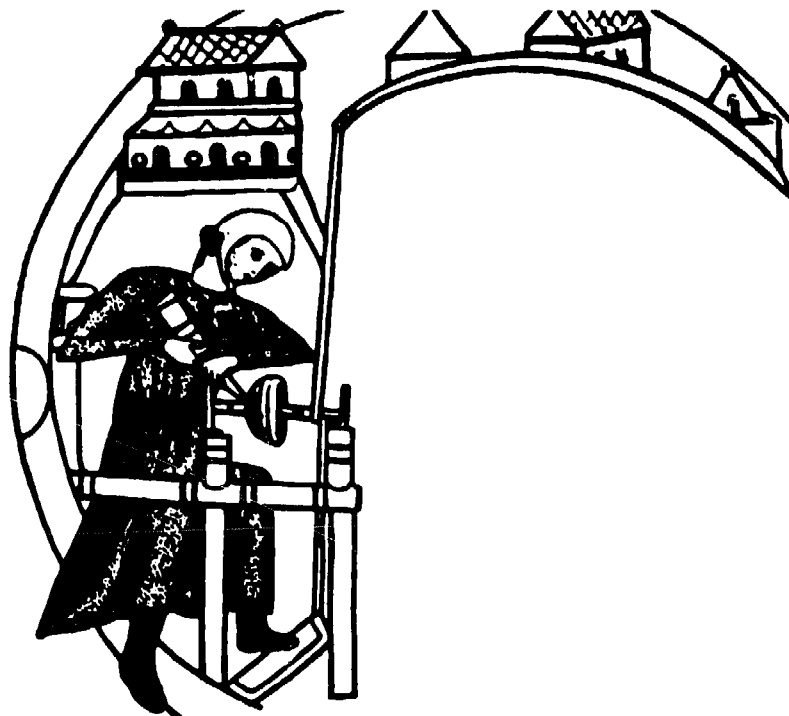
Figure 4.3 Bow-action lathe of the Middle Ages. Courtesy of Imperial Chemical Indus- tries, Ltd.
