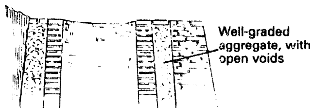
Insulating a hillside kiln.
