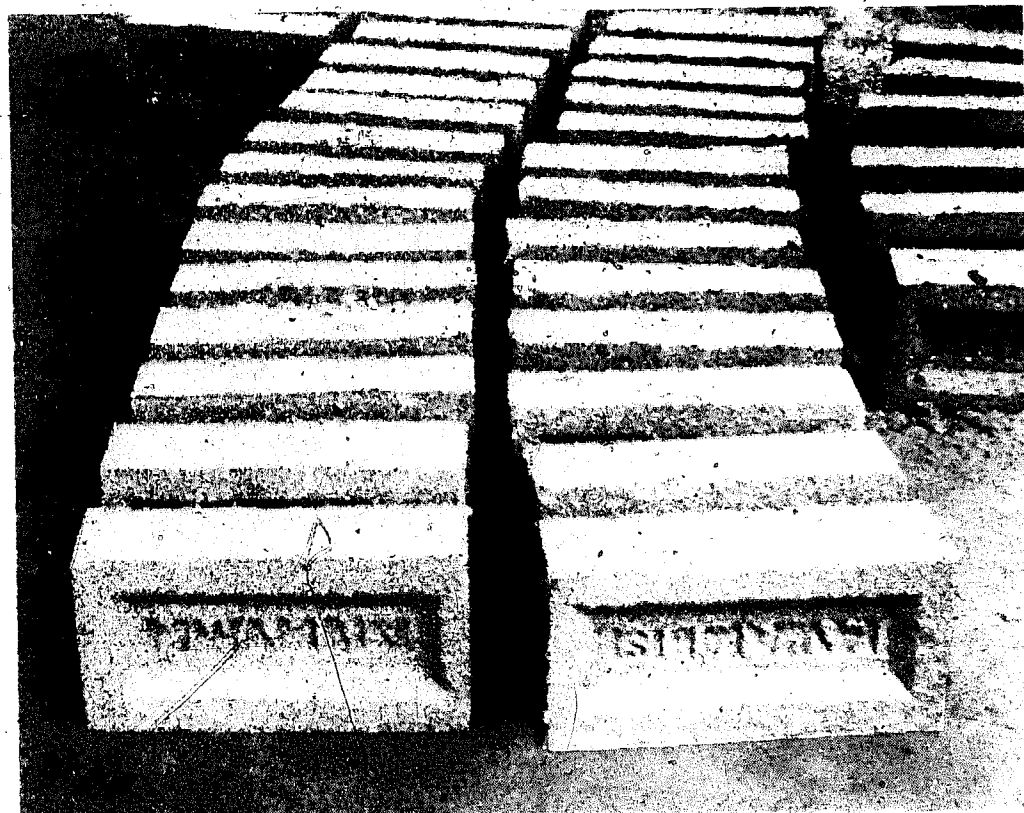
Sandmoulded bricks made in self-releasing moulds. Further development is now needed to obtain equivalent standard with slopmoulding system for locations where sand is not available
