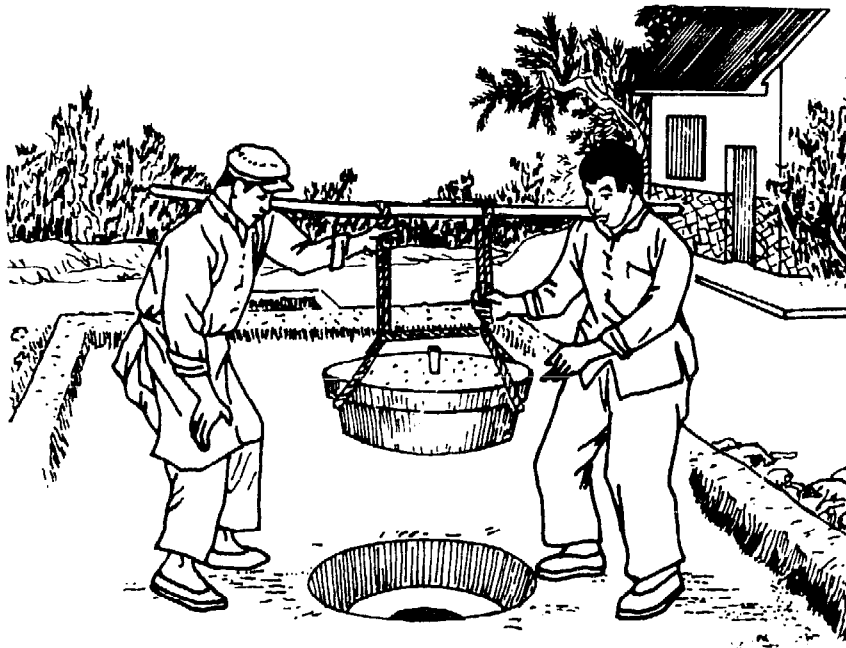
Fig. 4-23. Fitting a removable cover.
