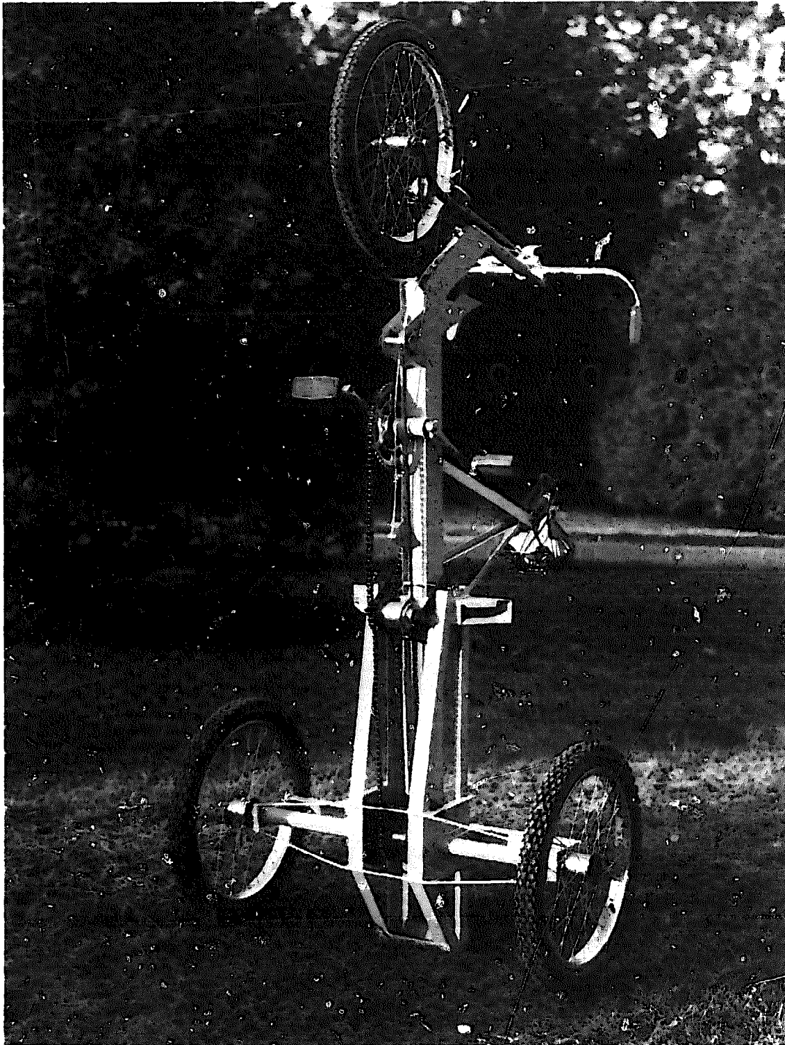
FIGURE 62 Up-ended view of the Oxtrike chassis, allowing ability to park in a small space, easy inspection of transmission and brakes, and ability to tip out the load. Note Sturmey-Archer three-speed hub gear with double adjustment for primary and secondary chains. (Reprinted from Pedal Power © 1977. Permission granted by Rodale Press, Inc., Emmaus, PA 18049)
