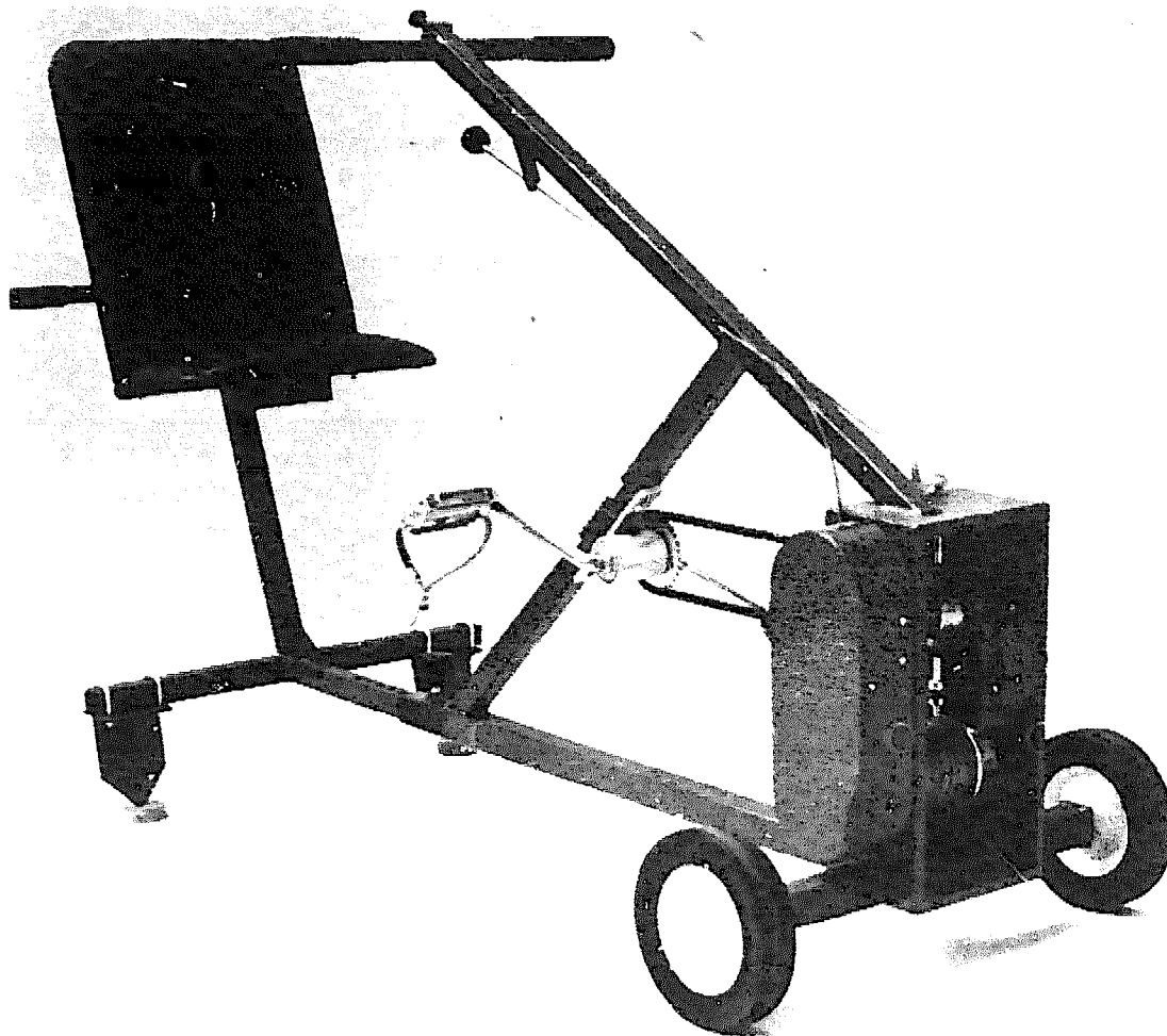
FIGURE 71 Pedal power winch unit of the Mechanical Mule™.
