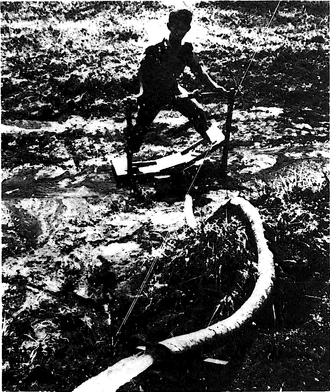
FIGURE 67 Pedal pump designed by the International Rice Research Institute, Los Baños, Laguna, the Philippines. (Reprinted from Pedal Power © 1977. Permission granted by Rodale Press, inc., Emmaus, PA 18049)
