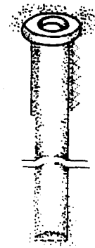
Bored Pit with Concrete Lining
