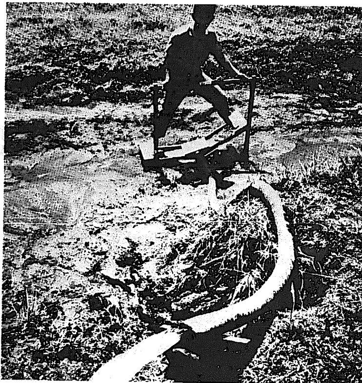
Fig. 3.15 Foot-operated bellows pump (Courtesy of IRRI)
