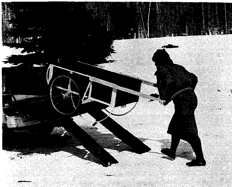
20. Flare boards as ramps.
