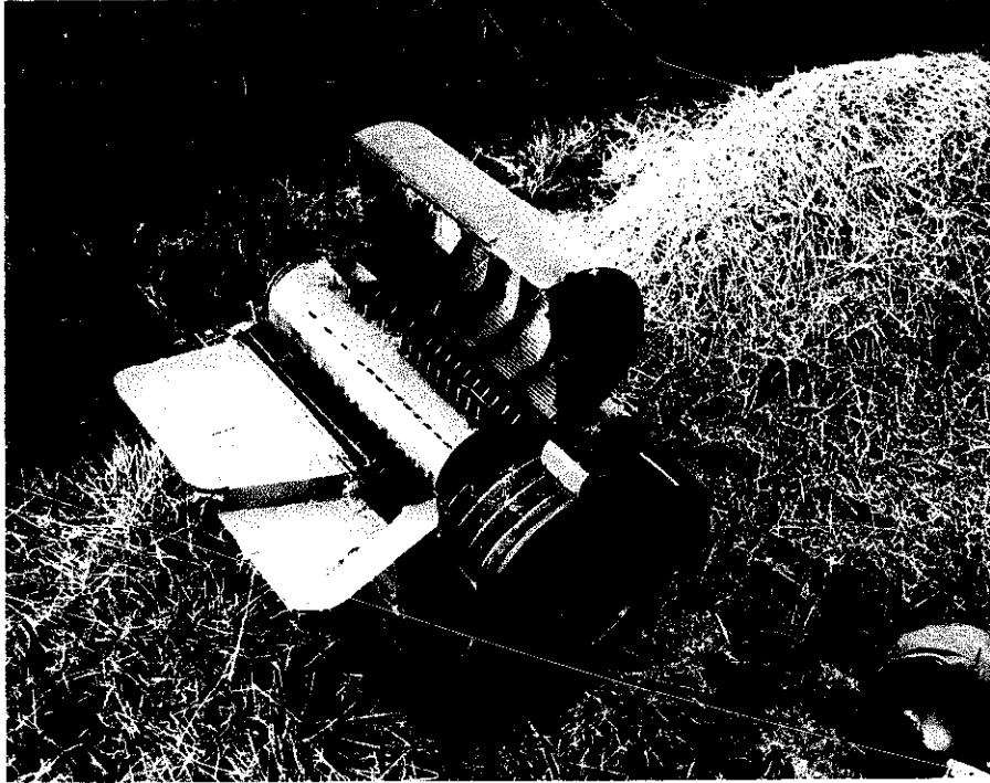
FIG. 53. Threshing cylinder and upper concave exposed in IRRI axial-flow thresher (courtesy IRRI).
